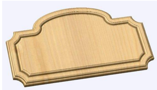
Profile Cutting Strategy with Form cutter
